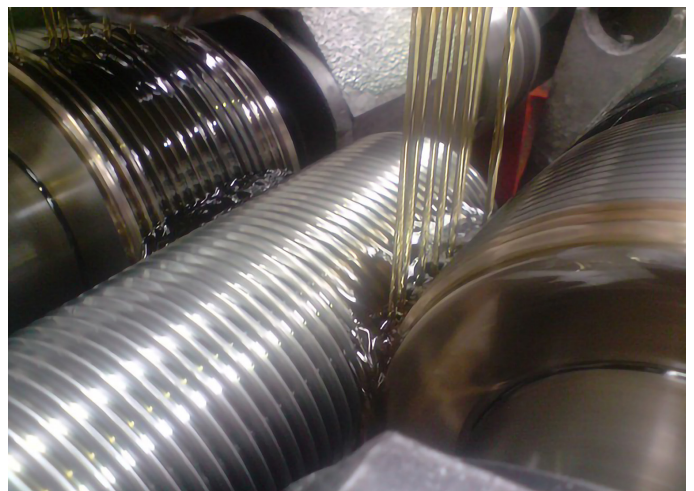
Threading M100 to BS3643.
